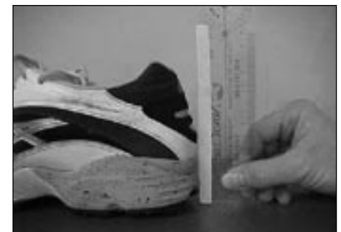
Figure 4. Qualitative assessment of the posterior heel flare for the Asics 126 (Asics Tiger Corporation; Irvin, Calif) running shoe. A straightedge is held perpendicular to the support surface against the most posterior aspect of the shoe. The anterior edge of the ruler makes contact with the posterior aspect of the heel counter just above the shoe's midsole material.
